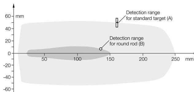
Detection range – using the M12 ultrasonic sensor (BUS M12E0...) as an example. Within range (A), the BUS sensor detects the standard target. Within range (B), the BUS sensor detects the standard target and the round rod.
