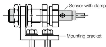
These aluminum mounting brackets provide a way of easily and quickly attaching sensors to the machine. When using tubular sensors, it is recommended that additional clamps be used.
