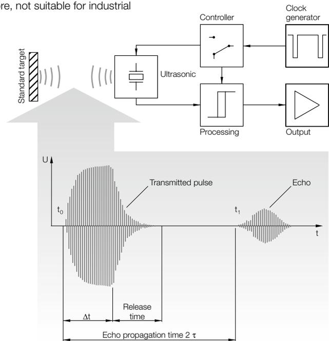
The range in which the sensor can detect objects is limited by the smallest and largest operating range. This, as well as the size of the blind zone, is determined by the size of the transducer. In the blind zone, the ultrasonic sensor cannot detect any objects. The zone is the result of the duration of the transmitted pulse and the release time of the ultrasonic transducer.
