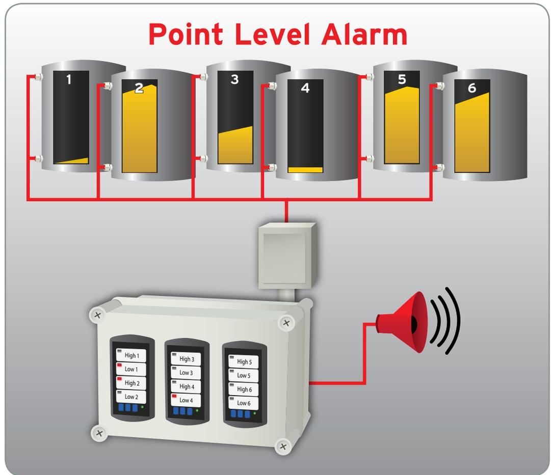
as a vessel is emptied or comes back into contact with the level indicator as a vessel is filled, the LED on the panel goes out altogether and the panel automatically resets – and is ready to receive the next alarm signal.
