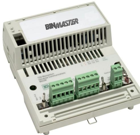
SmartBob II Momentum Universal Communication Module (MUCM) . The standard model allows Modbus serial masters to gather data from BinMaster SmartBob II remotes.
