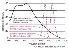
Use a camera sensitive in the near infrared region for use with an Infrared Light. The photographed image is affected by the distribution of the emission spectrum of the infrared LED and the spectral sensitivity characteristics of the camera. Optimized combination with an optical system is very important to achieve stable images.
