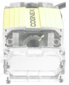
Tighten screws in order shown. Maximum torque for the cover screws is 9 N-cm (0.8 pound-inch).
