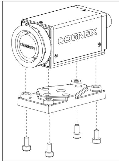
**Figure 2-1: Attach the Mounting Block**
