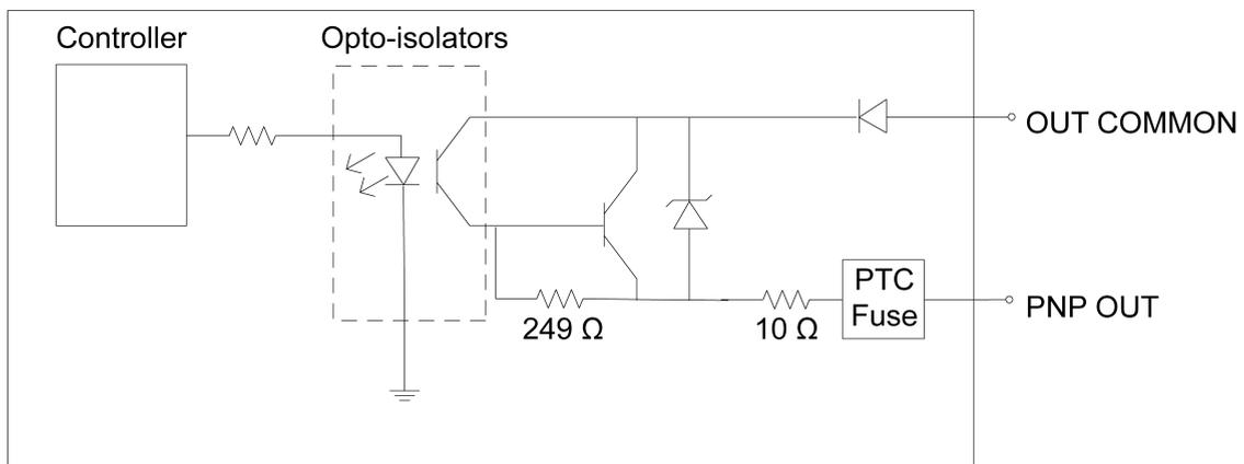
**Figure 3-3: PNP High-Speed Output Schematic**
