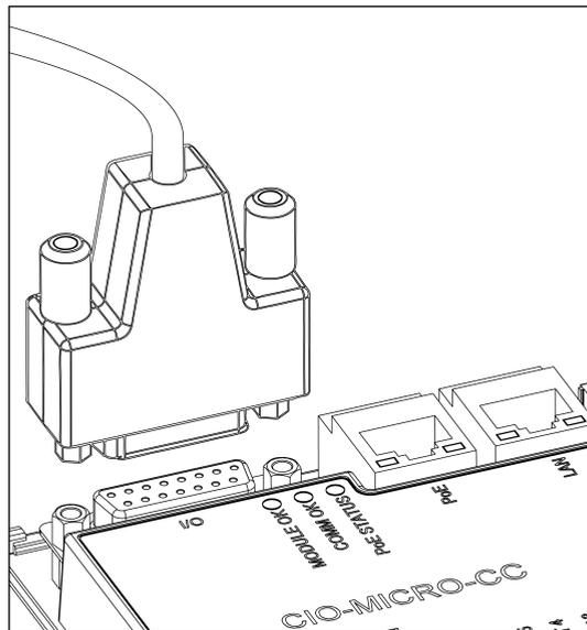
**Figure 2-5: Connect the I/O Module Cable to the I/O Module**
