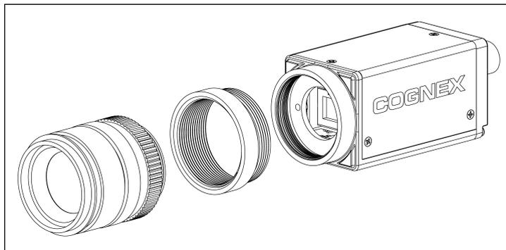
**Figure 2-2: Install the Lens (C-Mount with Extension Ring)**
