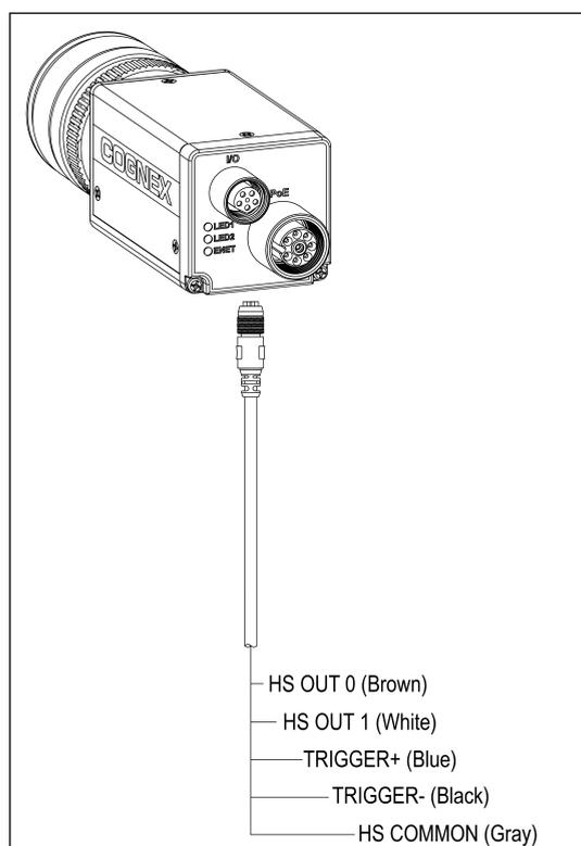
**Figure 2-3: Connect the Breakout Cable**
