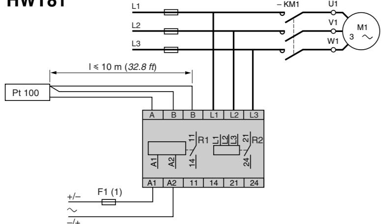
(1) 1 A fast-acting fuse. UL...Class CC ; IEC...gG
