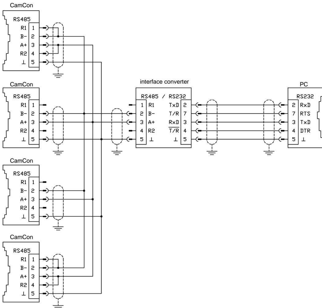
**Please note:** With an RS485 interface the connection plugs of the first and the last unit of a linked chain, pins 1 and 2, as well as pins 3 and 4 have to be bridged to close off the data and the input cable. Therefore the device has closedown resistors at pins 1 and 4.
