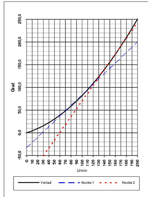
$$\text{Delay time ( in sec. )} = \frac{\Delta \text{ way (in } ^\circ \text{)} * 60 \text{ (sec./min.)}}{\Delta \text{ Speed (in rpm.)} * 360 \text{ (} ^\circ \text{/turn)}} = \frac{340-332 * 60}{40-30 * 360} = 0.133 \text{ sec.}$$
