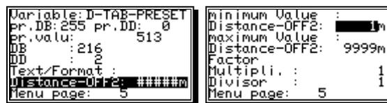
The "D-TAB-Preset" variables is used for simply feeding in parameters off an PLC-Logic-Module and needs 10 parameters itself:
