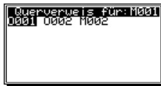
The register M001 is currently used in networks O001, O002 and M002.
