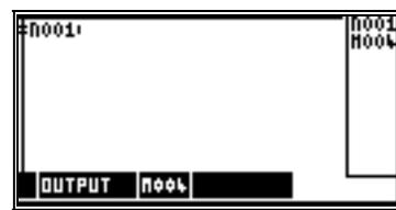
If the cam N001 is switched off (negative edge), the M005 flag is reset.
