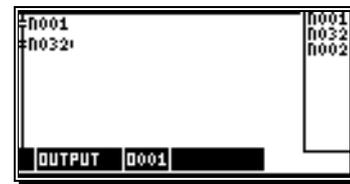
Output 1 of the CamCon is enabled when the rotation direction output 32 is **deactivated**.
