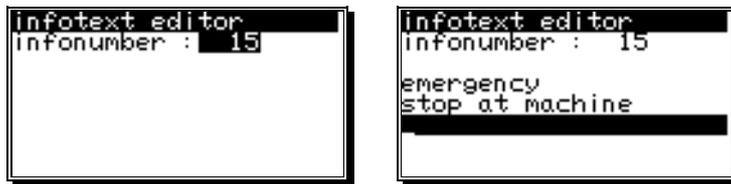
After confirming the message number ( Info number ) by pressing the **CR** key, you enter the input of the first text line (see chapter 7.2. Text input). There are 4 lines available with 21 characters each. If the first line is less than 10 characters, this line is later displayed in twice the normal height.
