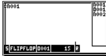
For the input of the message text the cursor has to be within the range of the function component, recognizable by the inverse display of the function component. By pressing the **#** key you initiate the input.
