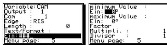
The variable "CAM" is used to enter cams and requires a total of 9 parameters:
