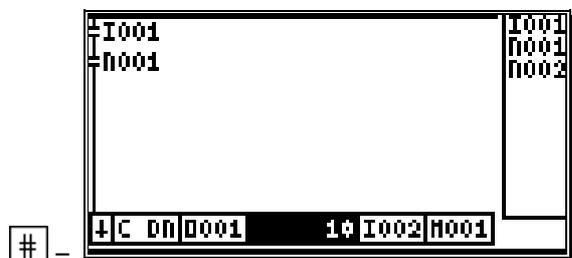
After the input of the counter value, that can be within the range of 0 to 9999999, the value is confirmed by pressing the  $\boxed{CR}$  key. After that you enter the input of the counter reset requirement.
