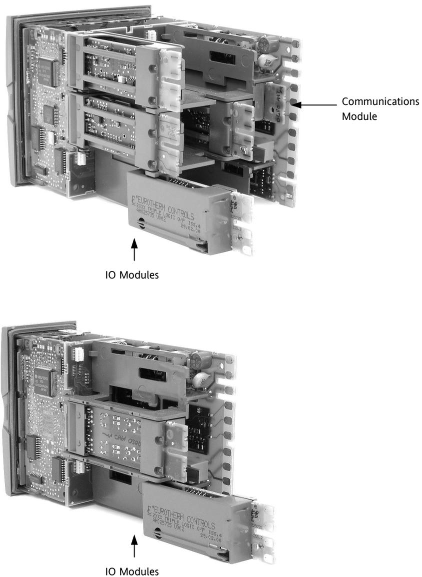
Figure 9-1: View of the Plug-in Modules
