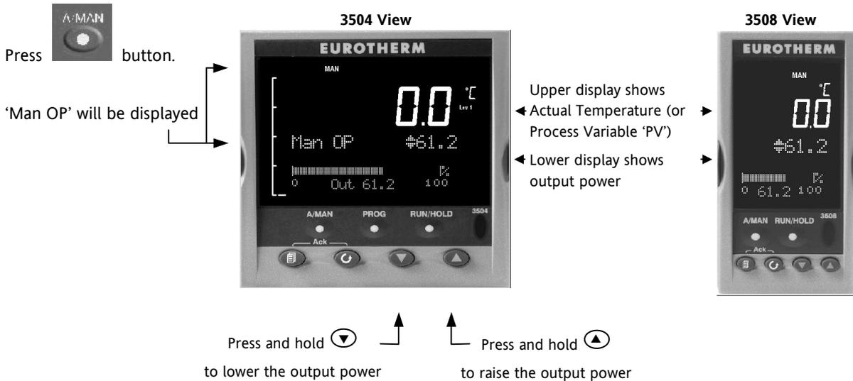
The output power will change continuously while either of these buttons are pressed
