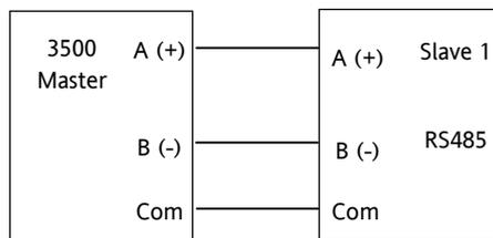
Figure 13-5: Rx/Tx Connections RS485 2-wire
