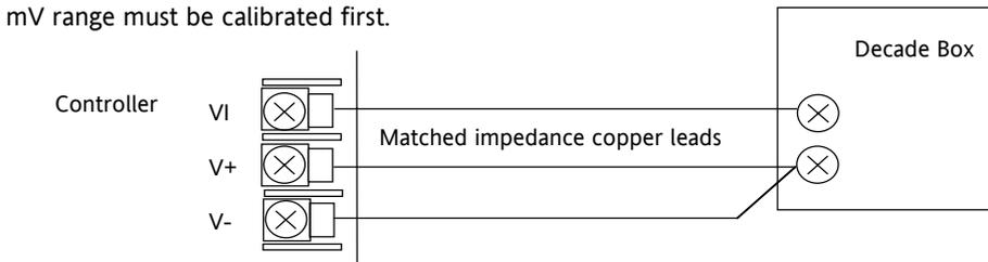
Figure 25-3: Connections for RTD Calibration
