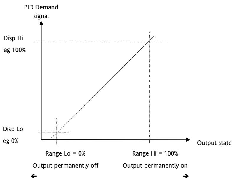
Figure 9-3: Time Proportioning Output
