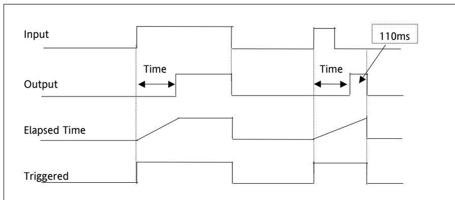
Figure 14-5: Off Delay Timer Under Different Input Conditions
