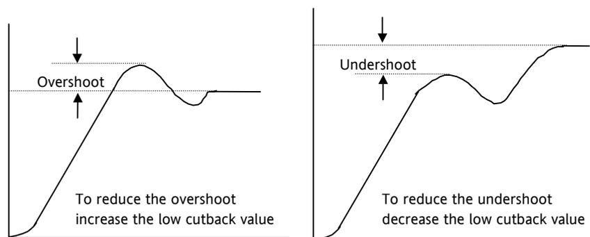
Figure 20-3: High and Low Cutback
