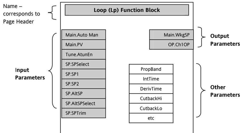
Figure 3-1: Example of a Function Block
