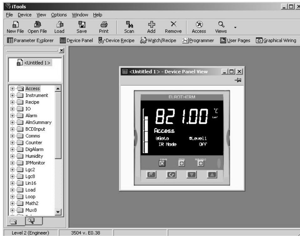
The front panel control buttons, shown in the Device Panel display, are active and clicking on them with the mouse will cause the display to behave as a real instrument.
