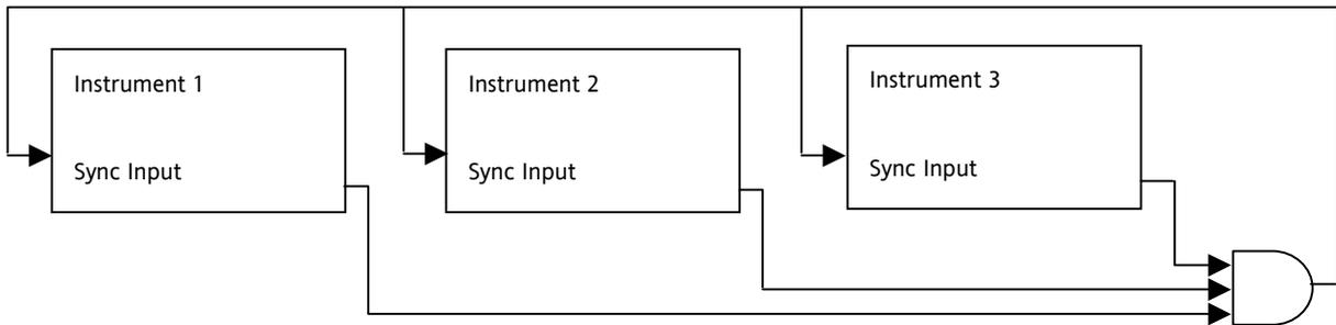
**Figure 21-5: Synchronisation of three controllers**
