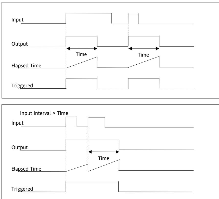
Figure 14-4: On Pulse Timer Under Different Input Conditions
