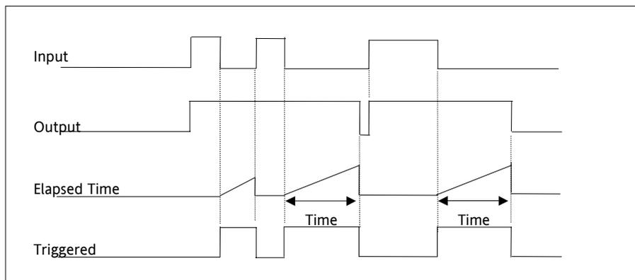
Figure 14-7: Minimum On Timer Under Different Input Conditions
