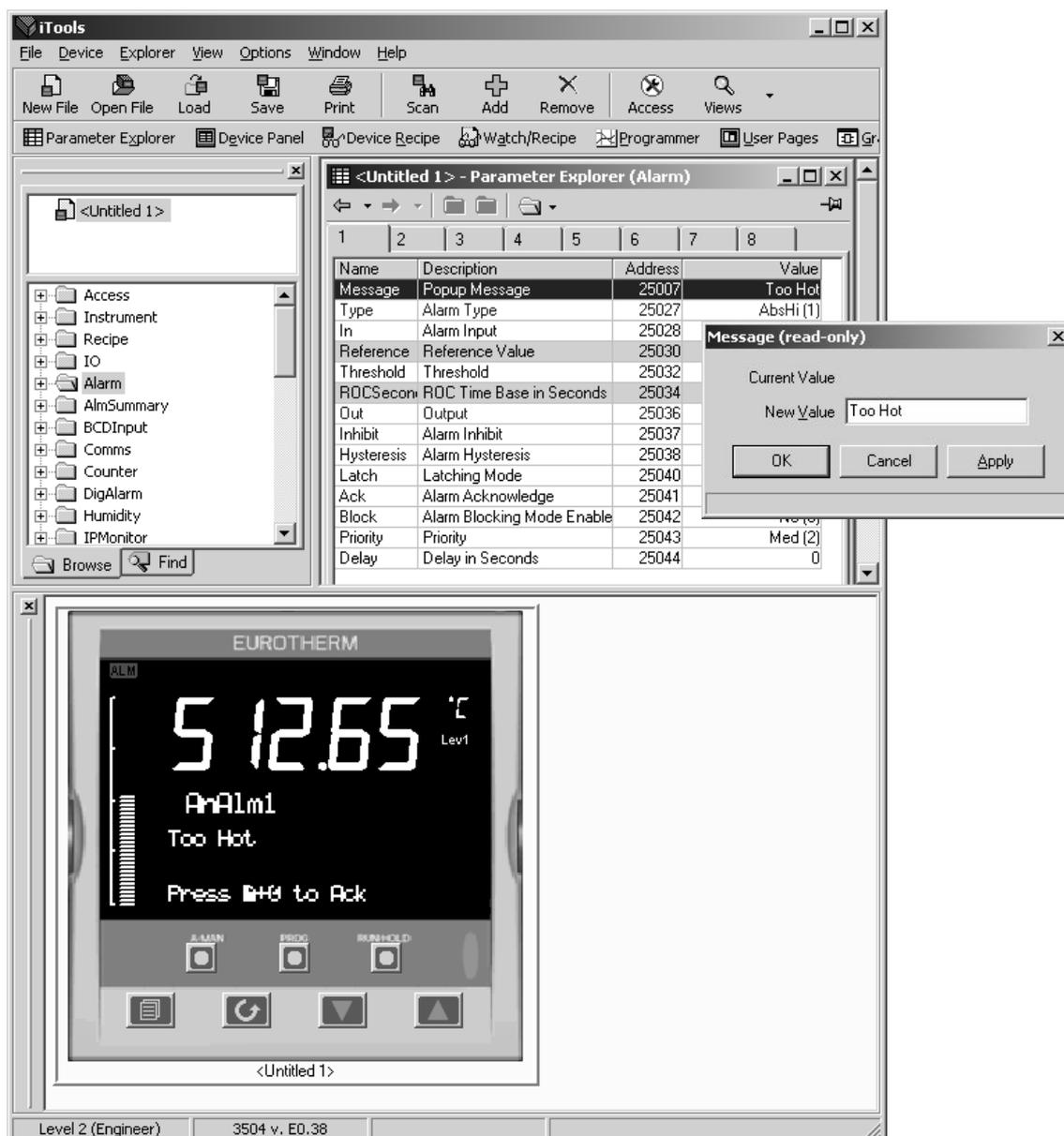
Figure 26-1: Configuring Analogue Alarms using iTools
