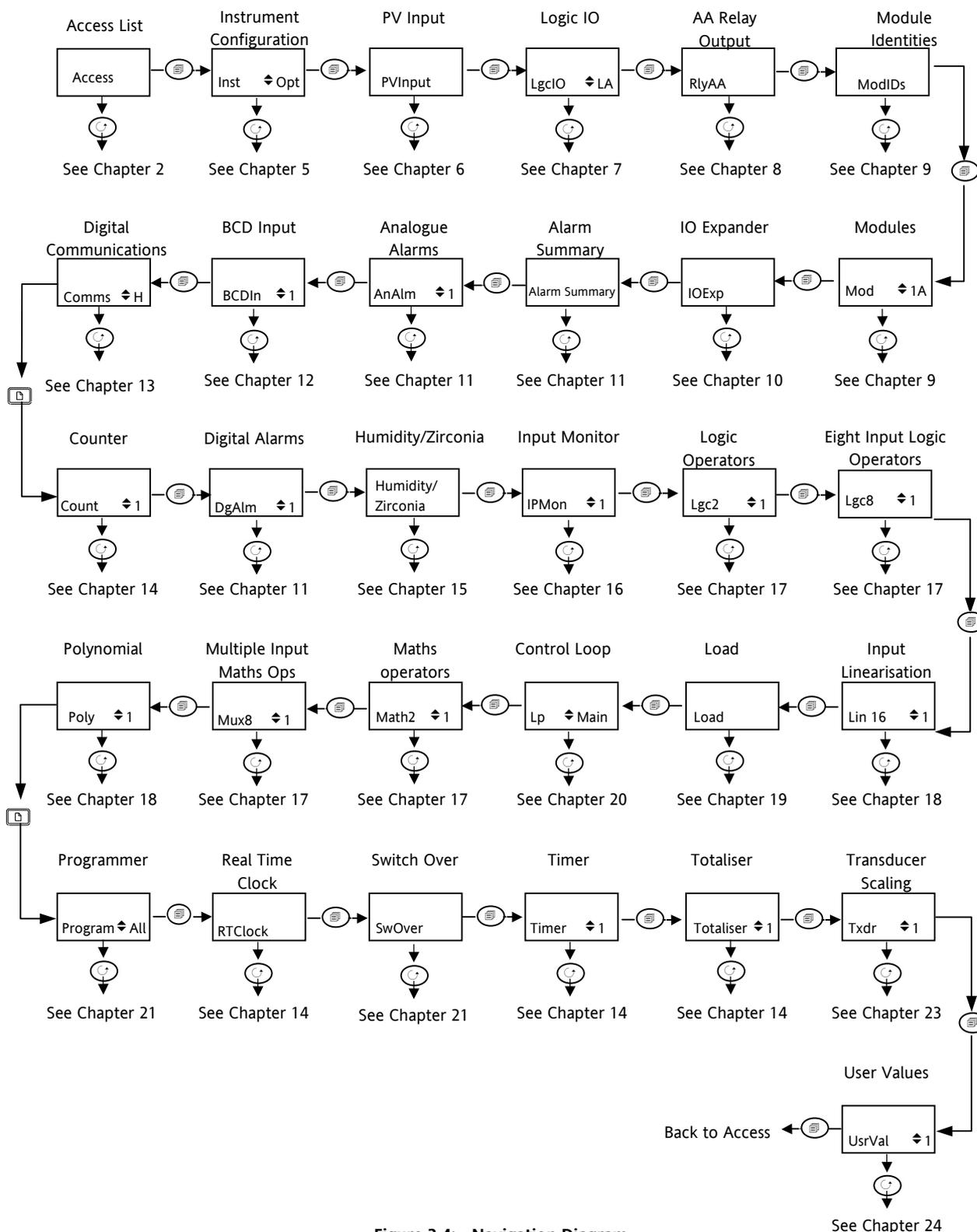
Figure 3-4: Navigation Diagram
