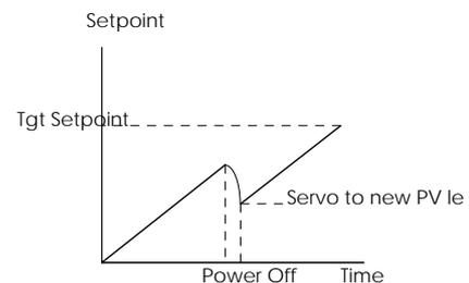
**21.1.12.3 Ramp back (power fail during Time-to-target segments)**
