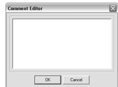
Comments can be linked to function blocks and wires. Hover the mouse over the bottom right of the comment and a chain icon will appear, click on that icon and then on a block or a wire. A dotted wire will be drawn to the top of the block or the selected wire segment.
