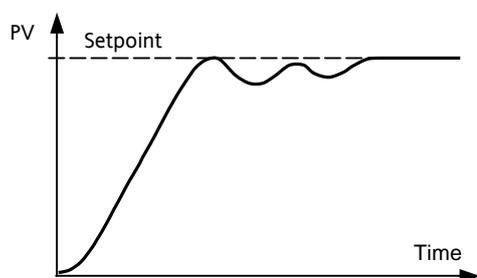
Autotune starts 1 minute after being turned on to determine steady state conditions.
