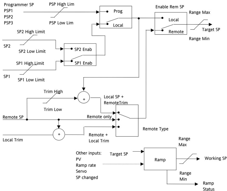
Figure 20-5: Setpoint Function Block
