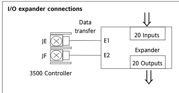
For details of the IO Expander refer to the Operating Instructions HA026893. The connections for this unit are reproduced below for convenience.
