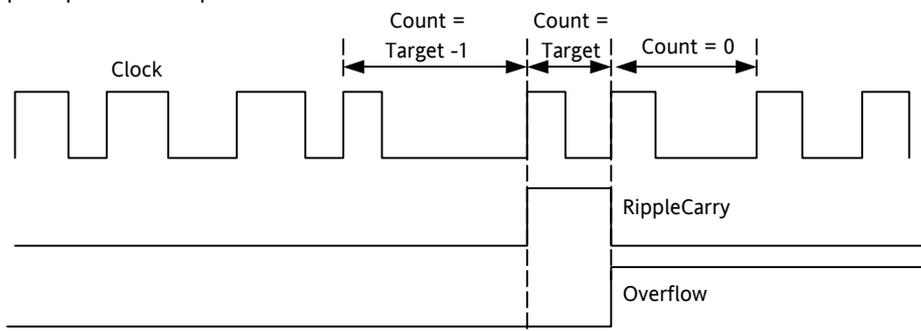
Figure 14-3: Timing Diagram for an Up Counter
