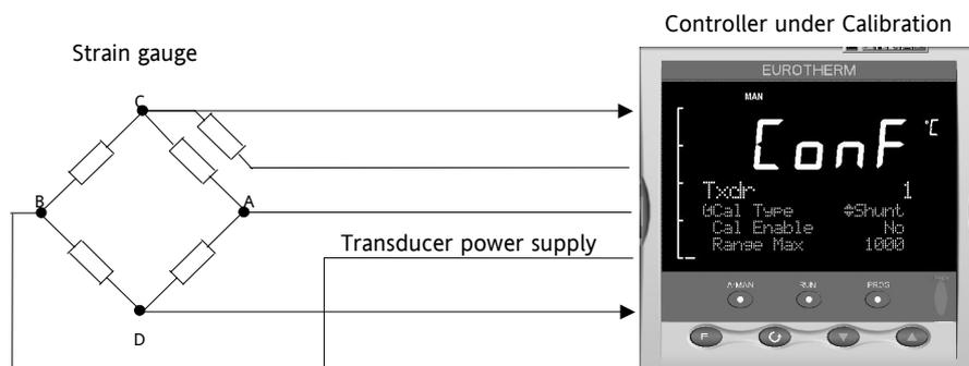
Figure 23-2: Strain Gauge
