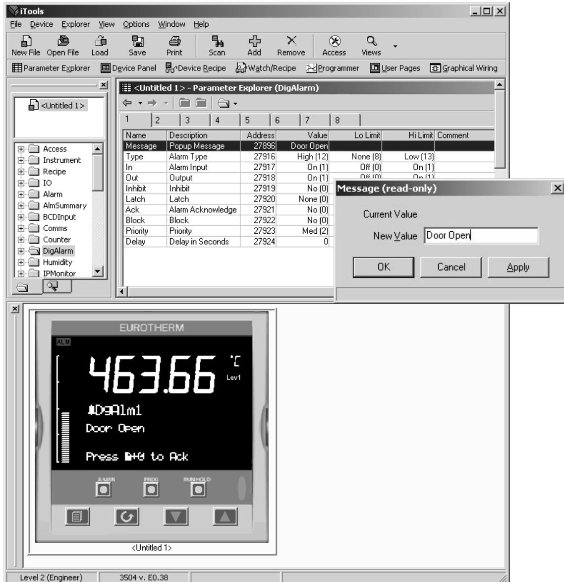
Figure 26-4: Configuring Digital Alarm Messages using iTools
