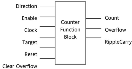
Figure 14-1: Counter Function Block
