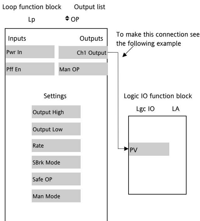
Figure 4-2: Function Block Wiring
