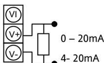
Connect the supplied load resistor equal to  $2.49\Omega$  for mA input
