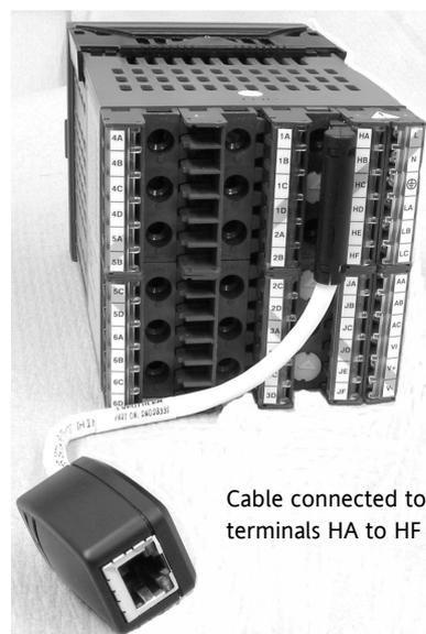
Cable connected to terminals HA to HF
