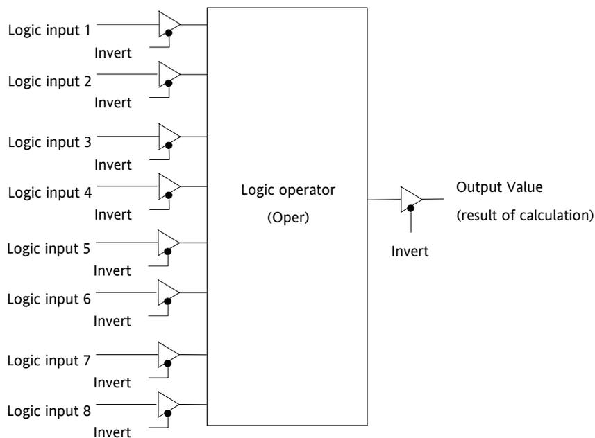
Figure 17-2: 8 Input Logic Operators
