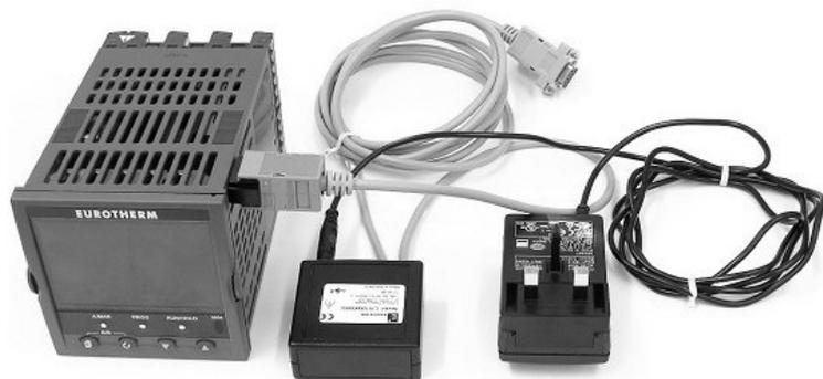
The DeviceNet communications module should not be fitted while using the CFG Clip as communications conflicts will occur. The minimum revision for DeviceNet communications module software used with the 3500 instruments is revision 1.6. This is identified by the module part no. AH027179U003.
