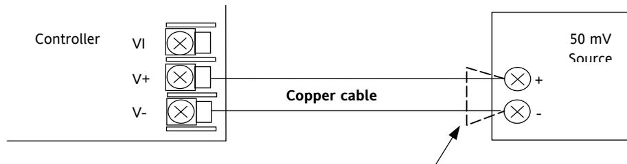
Figure 25-1: Connections for mV Input Calibration
