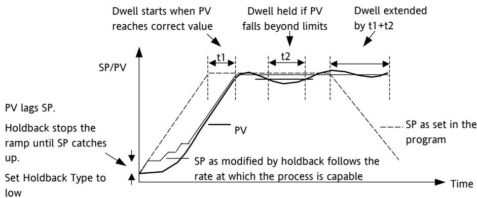
Figure 21-4: Effect of Holdback to Produce Guaranteed Soak
