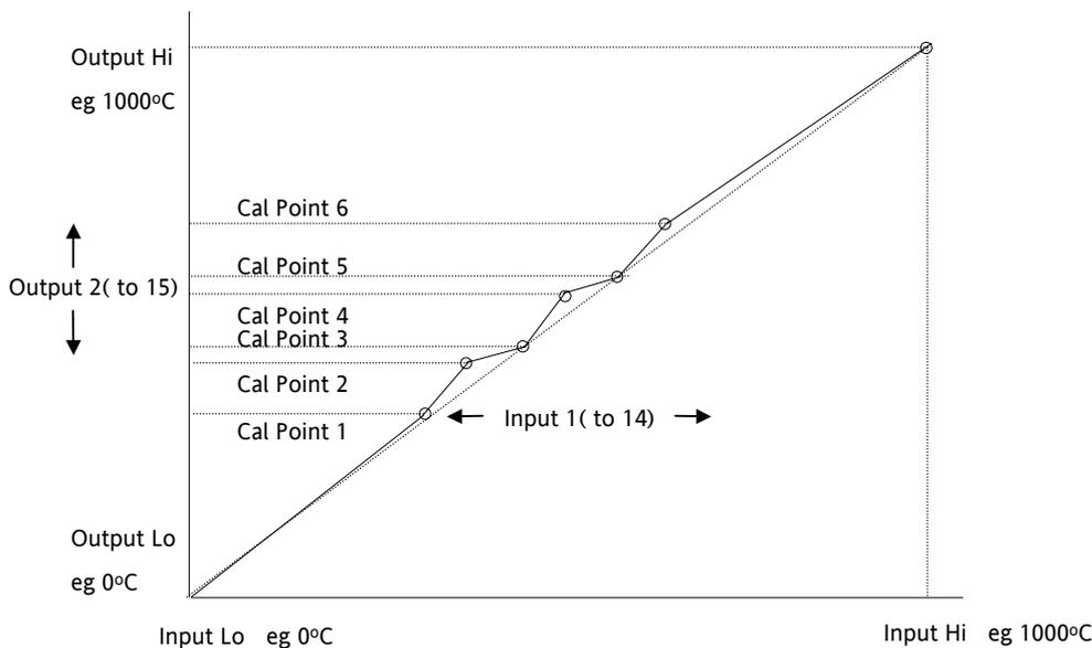
Figure 18-3: Compensation for Sensor Discontinuities
