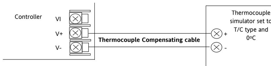
Figure 25-2: Connections for Thermocouple Calibration
