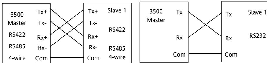
Figure 13-4: Rx/Tx Connections for RS422, RS485 4-wire, Rs232
