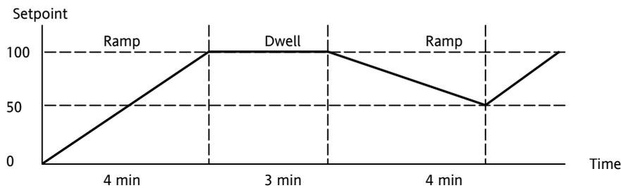
**Figure 21-2: Time to Target Programmer**
