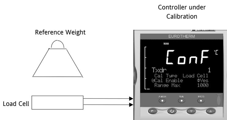
Figure 23-3: Load Cell Calibration
