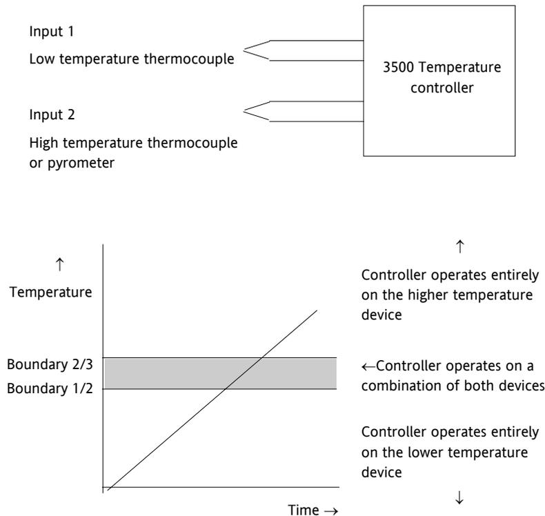
Figure 22-1: Thermocouple to Pyrometer Switching
