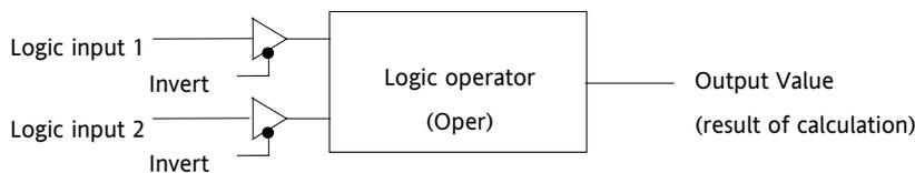
Figure 17-1: 2 Input Logic Operators
