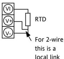
The resistance of the three wires must be the same
