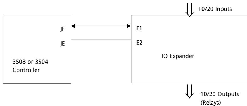
It is recommended that a cable length of 10 metres is not exceeded, however, no shielding or twisted pair cable is required.
