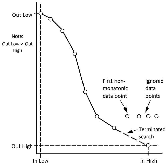
Figure 18-2: How an Inverted Curve will Terminate its search when it detects non-monotonic data
