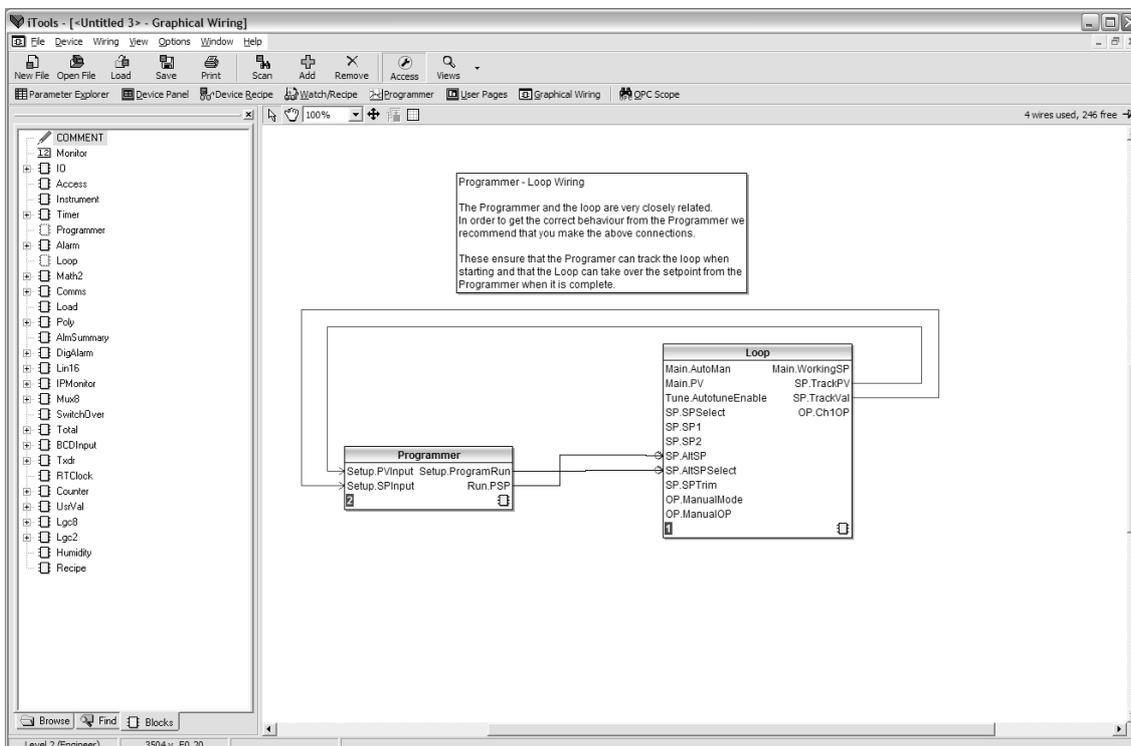
Note: The wires on this diagram are auto generated if the loop and programmer are enabled and there are no wires connected to the four inputs.
