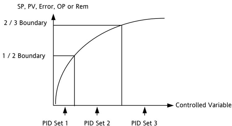
Figure 20-4: Gain Scheduling in a Non-Linear System
