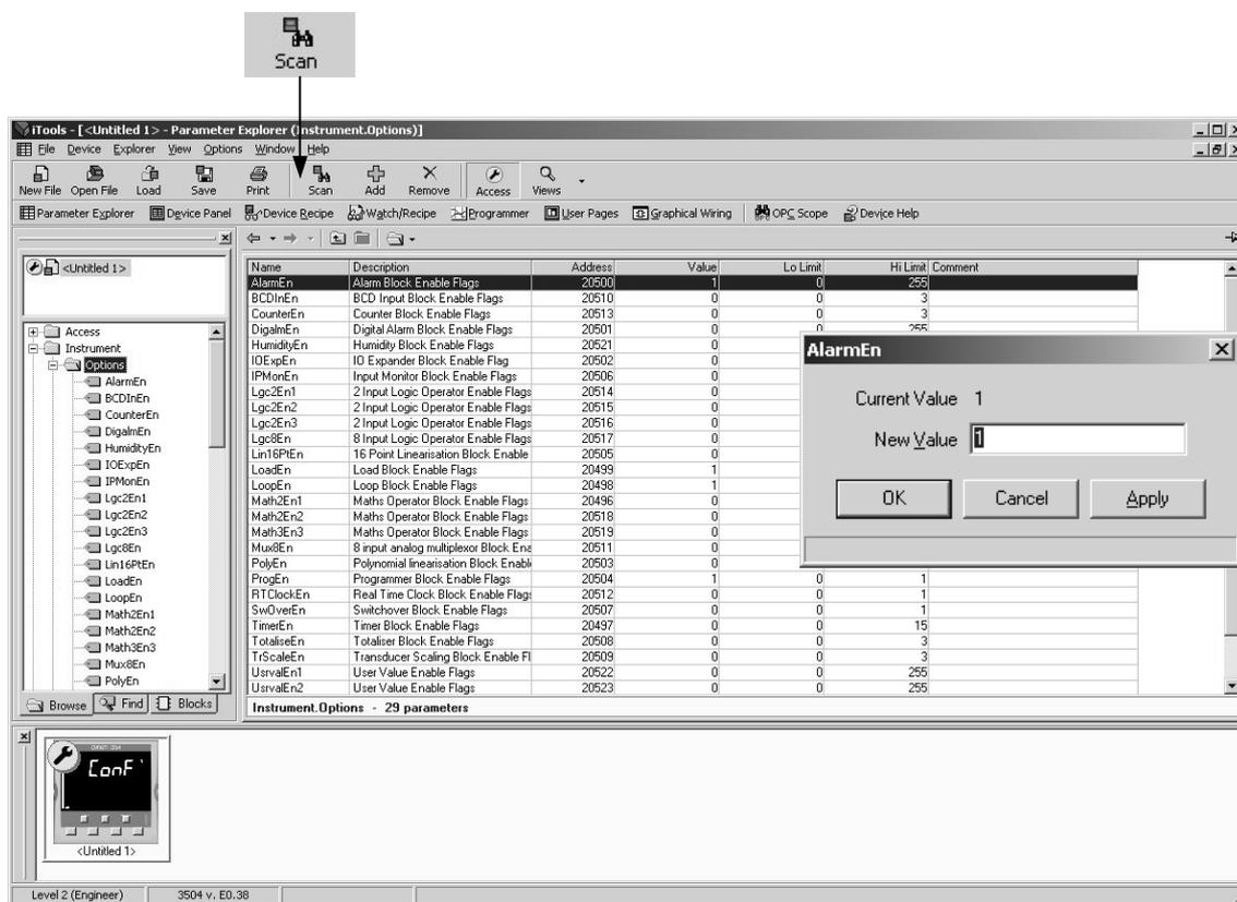
The example above shows how to enable an alarm
