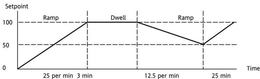
**Figure 21-3: Ramp Rate Programmer**
