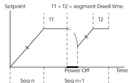
**21.1.12.2 Ramp back (power fail during Ramp segments)**
