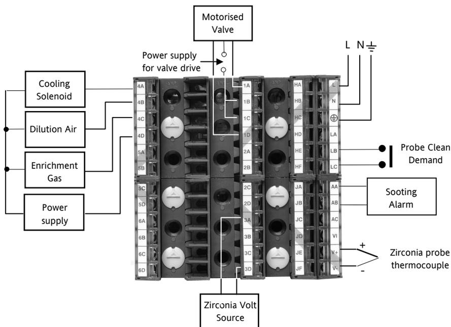
Figure 15-2: Example of Carbon Potential Controller Connections
