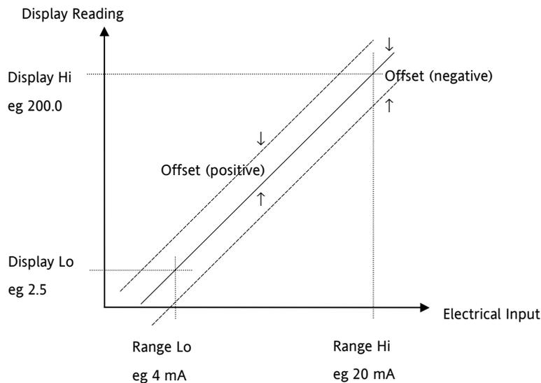
**Figure 9-2: Input Scaling (Standard IO)**
