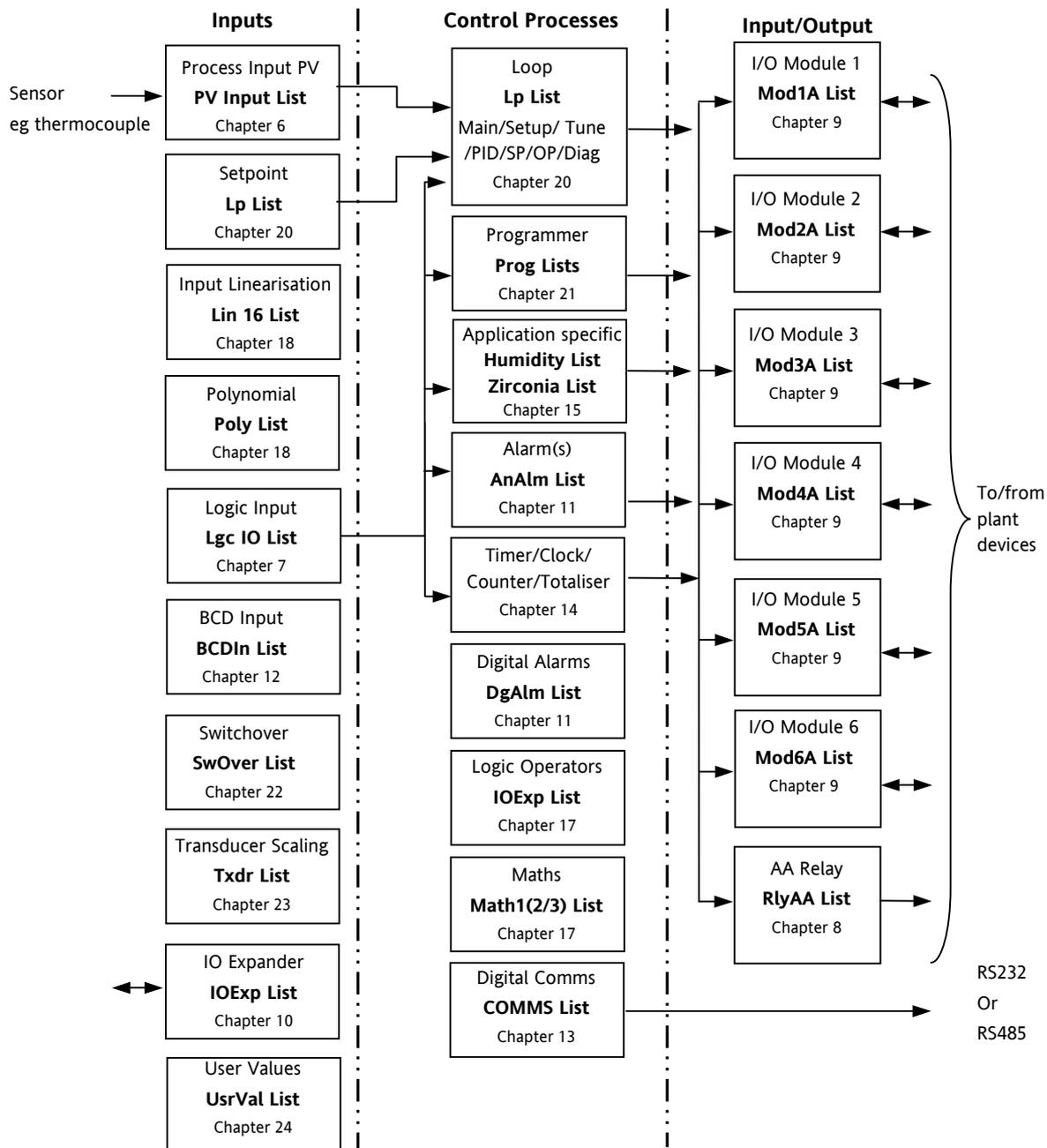
Figure 4-1: Controller Example
