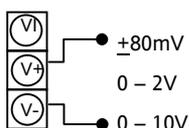
mV range  $\pm 40\text{mV}$  or  $\pm 80\text{mV}$
