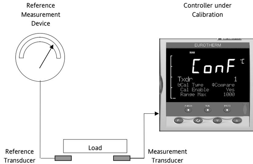
Figure 23-4: Comparison Calibration
