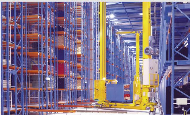
For positioning along the X- and Y-axes of high-bay storage devices and lifting gear, e.g. conveyor and storage technology (BPS 34/37), even with curves.
