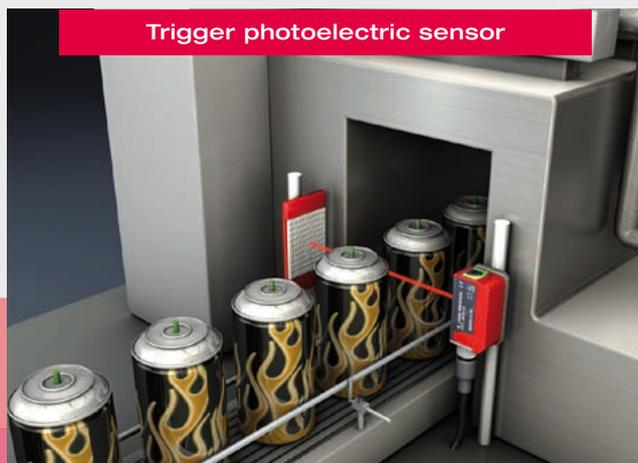
Trigger photoelectric sensor
