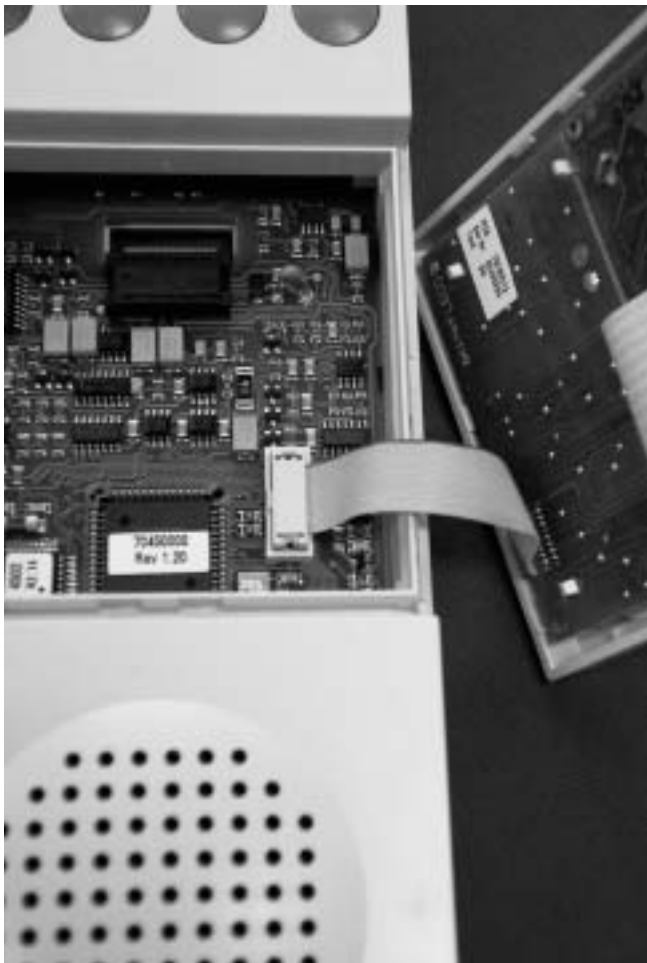
Communication-Terminal: Connection of Mother- and Daughter-Board with ODU MINI-FLAKAFIX
