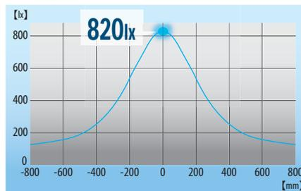
High power LED with 820 lx provides sufficient illumination with only a 174mA current draw.
