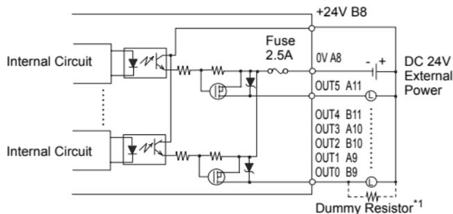
\*1 (Example) The output delay time (OFF to ON) is 1.5 $\mu$ s where the output current is DC 24V, 50mA. Install an external dummy resistor to increase the amount of current when more responsiveness is required and the load is light.
