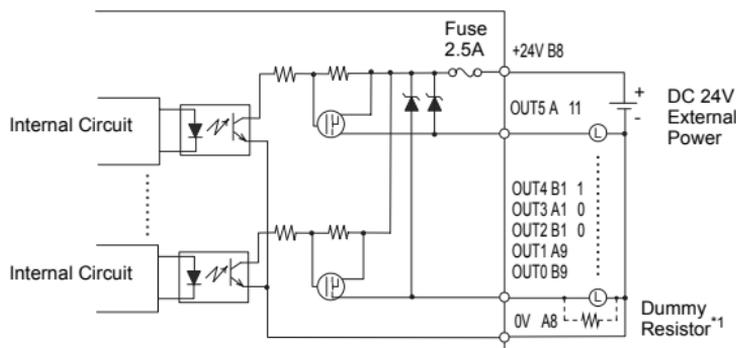
\*1 (Example) The output delay time (ON to OFF) is 1.5 $\mu$ s where the output current is DC 24V, 50mA. Install an external dummy resistor to increase the amount of current when more responsiveness is required and the load is light.
