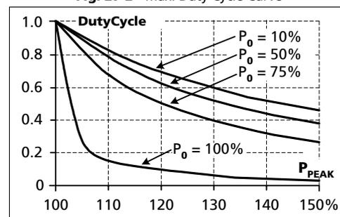
$$\text{DutyCycle} = \frac{T_{\text{peak}}}{T_{\text{peak}} + T_0}$$
