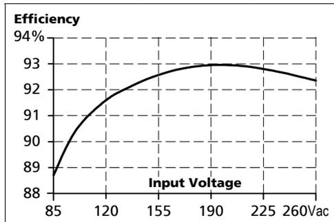
Fig. 11-4 Losses vs. input voltage, 24V, 5A
