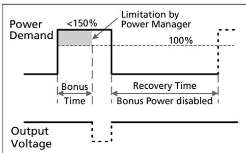
Bonus Power® is available as soon as power comes on and immediately after the end of an output short circuit.
