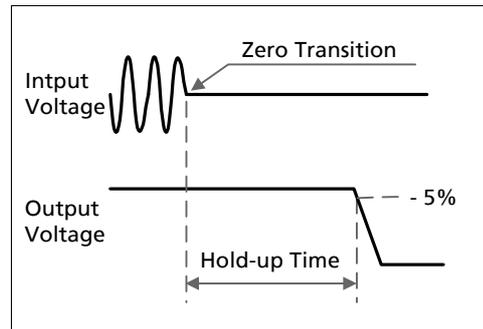
Note: At no load, the hold-up time can be up to one minute. The green DC-ok lamp is on during this time.
