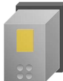
Drive mounted on a “footprint” filter
