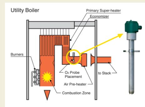
With the measurement of oxygen in the exhaust gas the flow of fuel can be controlled for optimum burner efficiency and minimum environmental effects.
