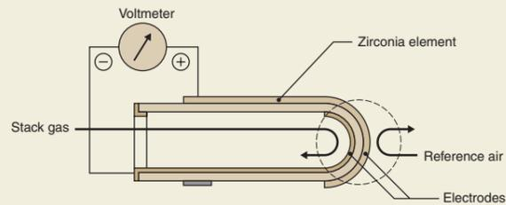
The principle of the zirconia oxygen analyzer is as follows:
