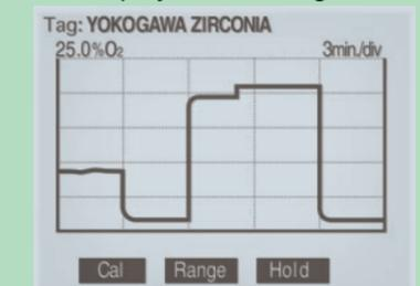
During automatic calibration, you can check stabilized display data while viewing oxygen trend data, thus providing highly reliable calibration.
